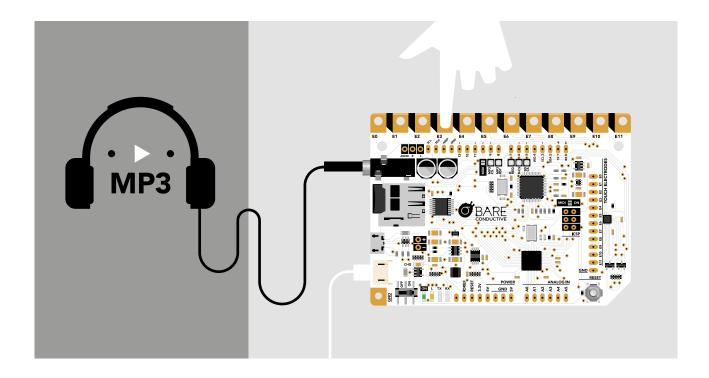
The Touch Board comes preprogrammed as an MP3 player complete with a micro SD card. This means that you can use it to trigger up to 12 MP3 tracks via touch, with no programming required.
