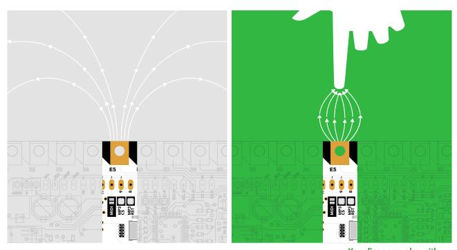
Each Touch Board electrode generates a sensitive electric field.
